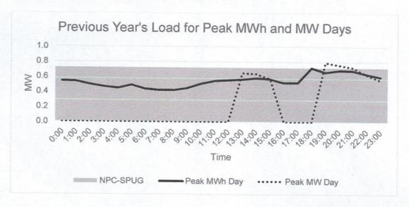
Peak MW occurred on 7:00 PM of April 28, 2023, while Peak MWh occurred on 6:00 PM of October 31, 2023 due to heavy usage of electricity on summer or dry season. As shown in the Load Curves, the available supply is lower than the Peak Demand.
