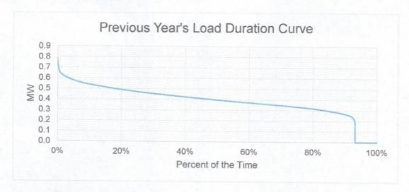
Based on the Load Duration Curve, the minimum load is 0 MW due to interruption in the area, and the maximum load is 0.795 MW for the last historical year.
