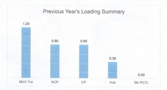
The Non-coincident Peak Demand is 0.80 MW, which is around 66.25% of the total substation capacity of 1.10 MVA at a power factor of 97.17%. The load factor or the ratio between the Average Load of 0.39 MW and the Non-coincident Peak Demand is 48.64%. A safe estimate of the true minimum load is the fifth percentile load of 0 MW.
