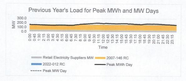
Peak MW and daily MWh occurred on 10:55 AM of July 7, 2023. As shown in the Load Curves, the available supply is lower than the Peak Demand.
