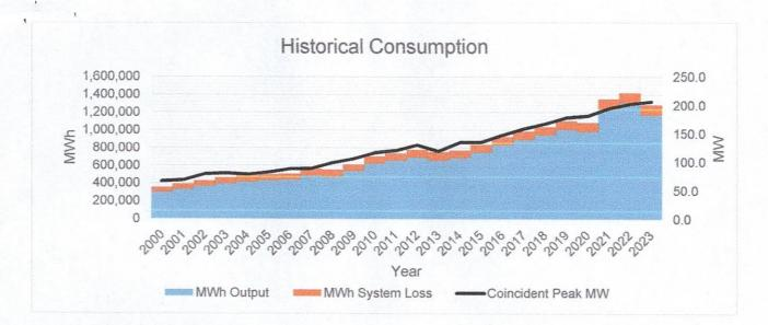
MWh Output decreased from year 2022 to year 2023 at a rate of 10.60%, while MWh System Loss decreased at a rate of 0.34% within the same period.
