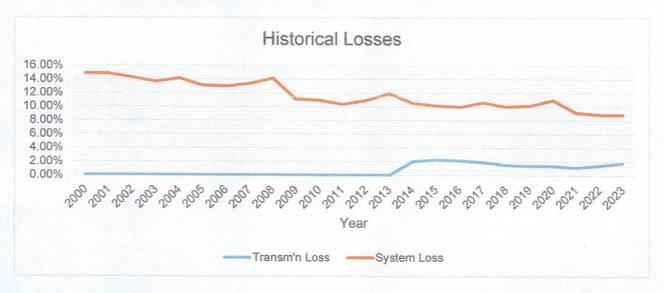
Historically, Transmission Loss ranged from 1.15% (2021) to 2.31% (2015) while System Loss ranged from 8.88% (2023) to 14.82% (2000). Transmission Loss peaked at 2.31% on year 2015 because it was the first whole year transition period of BATELEC II with customer under Retail Electricity Supplier (RES). System Loss peaked at 14.82% on year 2000 because of pilferages and other technical losses such as lengthy lines, existing old meters and equipment, inadequate size of conductors and etc.
