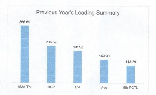
The Non-coincident Peak Demand is 236.57 MW, which is around 64.71% of the total substation capacity of 365.60 MVA at a power factor of 96.36%. The load factor or the ratio between the Average Load of 149.90 MW and the Non-coincident Peak Demand is 72.44%. A safe estimate of the true minimum load is the fifth percentile load of 113.29 MW which is 47.89% of the Non-coincident Peak Demand.
