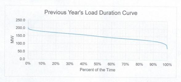
Based on the Load Duration Curve, the minimum load is 73.2432 MW and the maximum load is 206.9206 MW for the last historical year.
